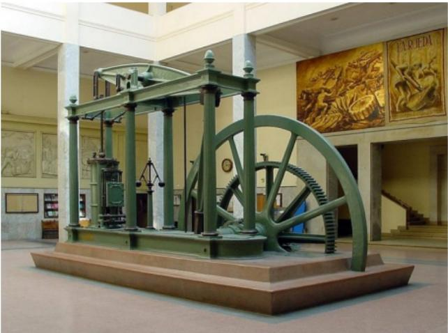
Source: Wikipedia, A late version of a Watt double-acting steam engine, built by D. Napier & Son (London) in 1859 ... Steam engines of this kind propelled the Industrial Revolution in Great Britain and the world.
